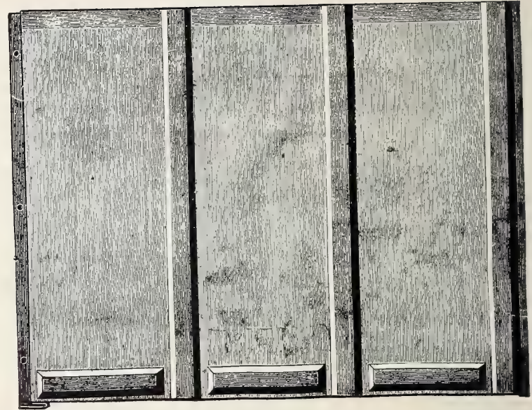
No. 701 —Shows our Manitoba pattern of siding made with telescopic side lock, which is created for use more especially on the sides of elevators. By its construction it is possible to apply it to an elevator or any other style of building liable to settle, so nailing it that it will settle with the building, thereby preventing the sheets buckling. It is shipped from our factory dipped in a coat of best oxide of iron paint mixed with pure linseed oil and all ready to apply on arrival.
